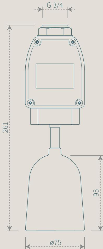
Assembly by tube suspension with threaded end G 3/4.
